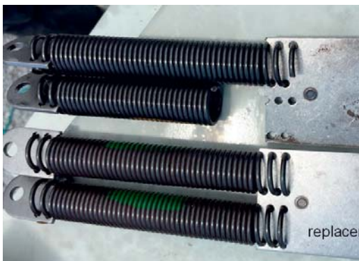
Figure 11. Broken spring assembly and replacement set
